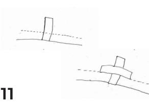
Cut three lengths of rope each approximately 150 cm long. Place tape for reinforcement in the middle of each of the edges of the opening. Then punch a hole through each of them above the rope reinforcement you created in step 5.
