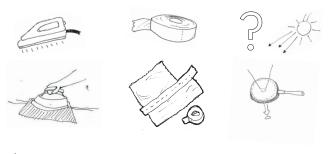
You can use different methods to connect two plastic bags to each other. One option is using a hot iron along the seam of two overlapping plastic sheets. Remember to place tissue paper on top of the surface to avoid melting of the plastic. Alternatively you can place tape along the seam. And maybe you could even invent a converging lens to fuse the plastic together?
