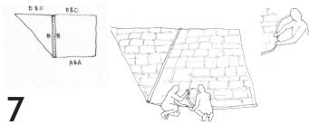
Tape the other pair of sides corresponding to A-A in the preceeding diagram. Carefully fold the tape over the edge, pressing firmly to achieve a strong, reliable connection.
