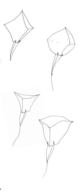
Only after you have flipped the structure inside out, tie the three ropes together and then attach a longer piece of rope to the connection....
