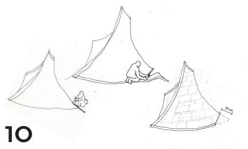
Flatten the structure around one of the corners. Your choice of corner will influence the final shape. Measure out 20 cm from corner on both of the edges. Mark the points and connect them. Cut a straight line.
